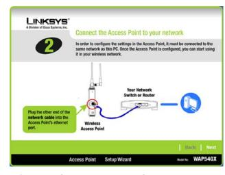
Figure 5-3: Connect the Network Cable to the Access
